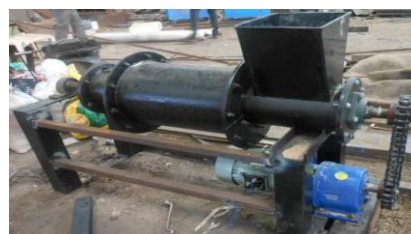
Fig.1 Experimental setup of Agro Waste Briquettes making machine
